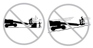
Limit travel speed according to the condition of the ground surface, congestion, slope, location of personnel, and any other factors which may cause collision.
