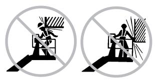
Be aware of crushing hazards when grasping the platform guard rail.
